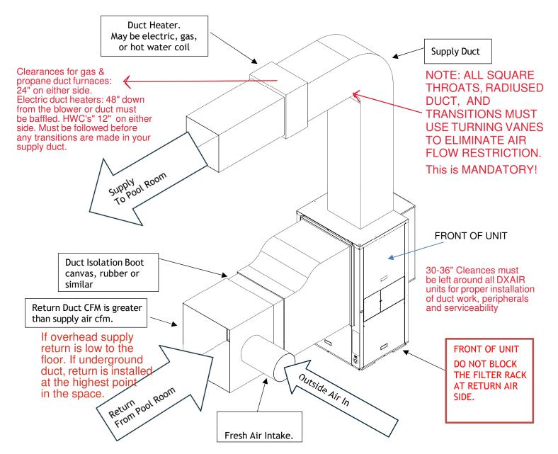
Underground ducting is installed at a slight pitch back towards the floor drain. Connections are under the return air side of the unit.
