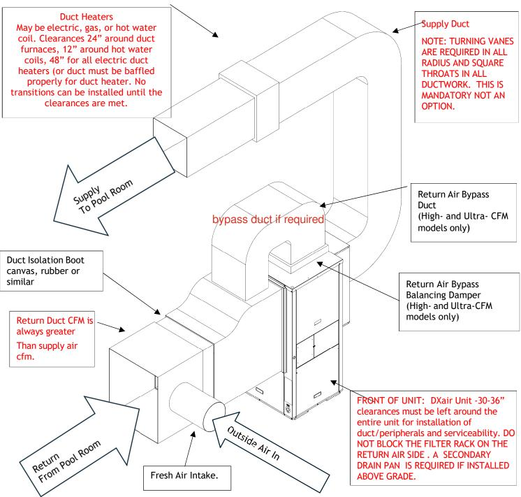
Example: High CFM Unit Bypass is required. Example: Horizontal Supply
