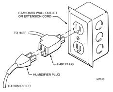
Fig. 3. Connecting H46F interrupter plug.
