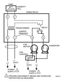
Fig. 6. Typical wiring diagram for H46D with a switching relay.
