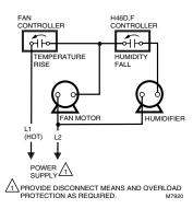
Fig. 4. Typical wiring diagram for H46D,F single-speed fan motor.
