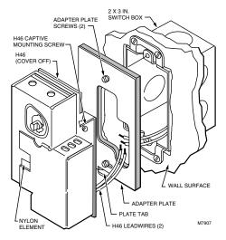
Fig. 1. Mounting H46D on vertical switch box.
