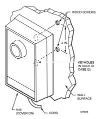
Fig. 2. Mounting H46F with two screws.
