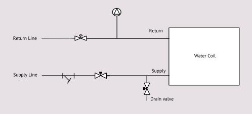
FIGURE 2. PIPING FOR WATER COIL
