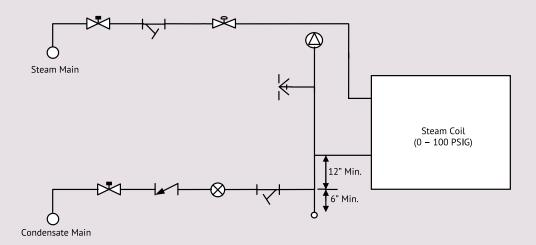
FIGURE 1. PIPING FOR STEAM COIL
