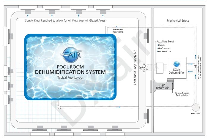
**NOTE:** Example Drawing only not to scale. This example is underground ducting with a high return air. Overhead ducting would utilize a low return air. Note all diffusers are deflected at all glass surfaces to move warm air and prevent condensation. DXAir will provide engineering and shop drawings for the air delivery system for your project.
